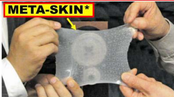
*EMBEDS INSIDE SILICONE SHEET ROWS OF SPLIT-RING RESONATORS CONTAINING LIQUID METAL ALLOY GALINSTAN MADE OF GALLIUM, INDIUM, TIN. (PROF. JIMING SONG & ASSOC. PROF. LIANG DONG OF IOWA STATE UN.)
